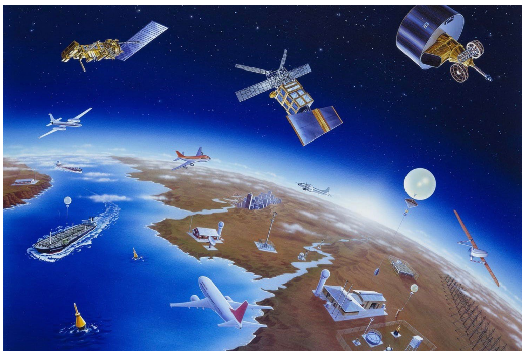
THE WMO INTEGRATED GLOBAL OBSERVING SYSTEM (WIGOS). Satellite observations, including those that use passive sensing techniques in radio frequency bands, are a crucial part of the WMO Integrated Global Observing System (WIGOS) used to support numerical weather prediction. (Source: WMO)
