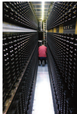
ECMWF's new automated tape libraries (ATLs) during construction. Each ATL from Sun can host 10,000 one-terabyte tape cartridges. Photographs, Neil Storer, ECMWF.
