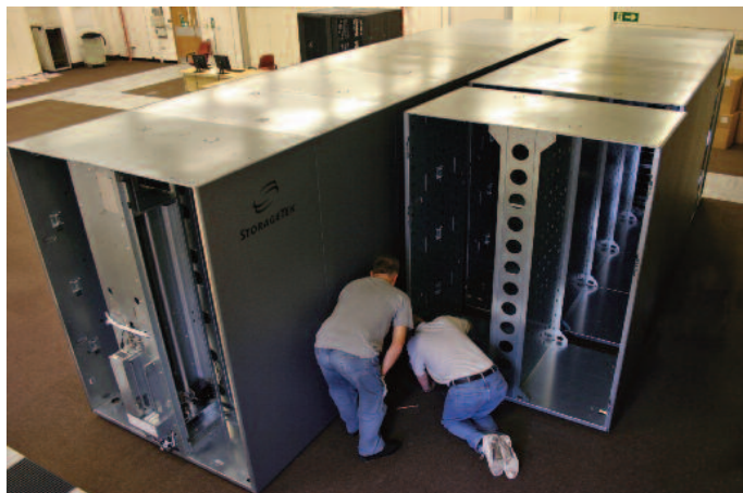
ECMWF's new automated tape libraries (ATLs) during construction. Each ATL from Sun can host 10,000 one-terabyte tape cartridges. Photographs, Neil Storer, ECMWF.
